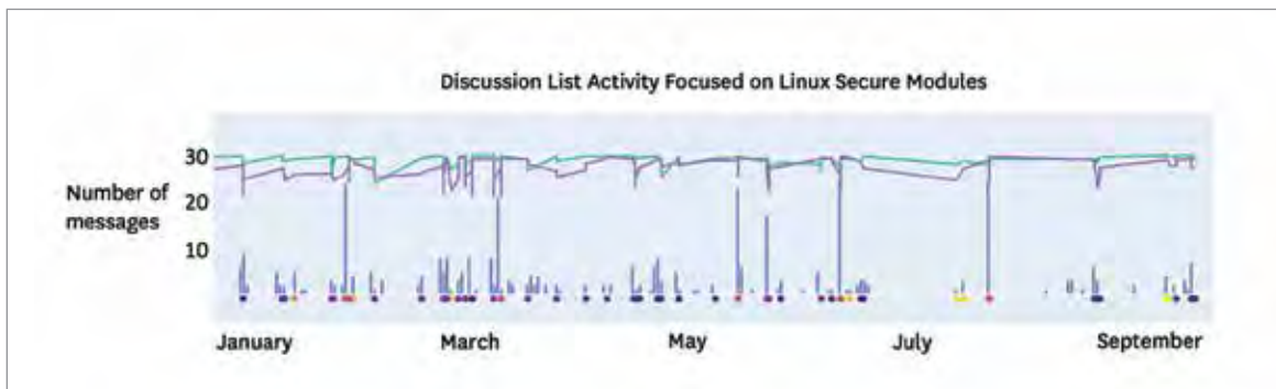
Part of the SACHET dashboard, this view shows recent activity in the subtopic of Linux Secure Modules (LSM). The bars show the total number of messages in a day, and the dots below are color-coded to individual developers who submit patches. The lines above show changes from the previous five patches, of authors (green) and of files affected (purple). The bursts in activity that coincide with such a change in focus in June and July show the introduction of the new AppArmor module.
